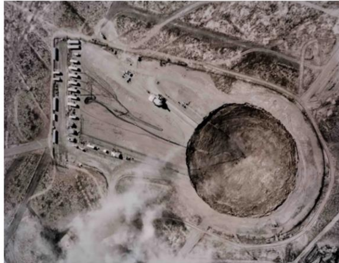
An aerial view of the subsidence crater formed by the Huron King underground nuclear test in Nevada on June 24, 1980. (FPG/Archive Photos/Getty Images)
