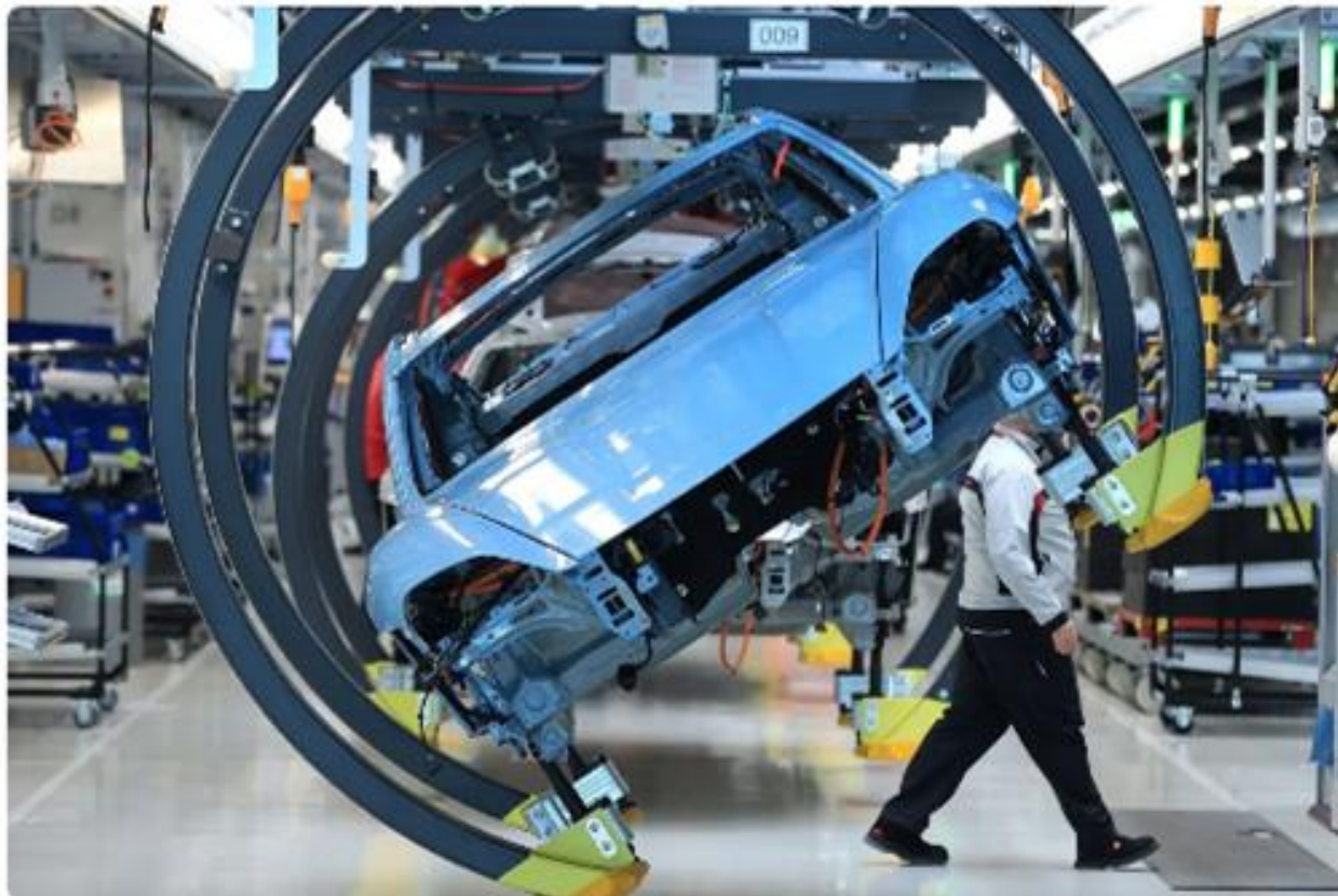
Body shell of an all-electric Porsche Taycan luxury automobile in an overhead conveyor cradle on the production line with man walking behind
